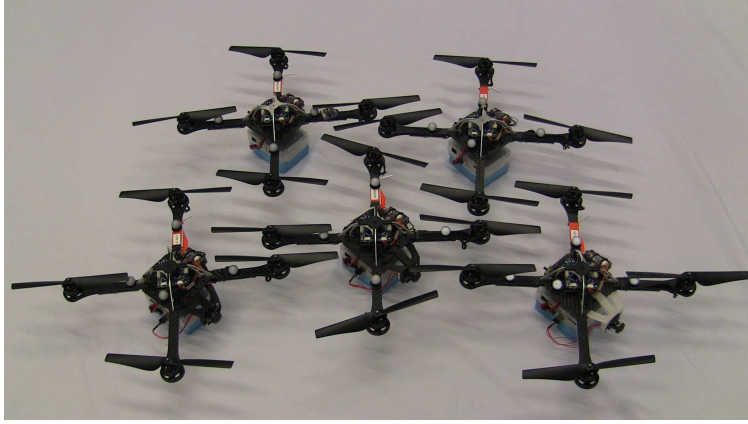
(b) AscTec Hummingbird quadrotors. Each quadrotor carries an ODROID XU3 computer with a wireless ethernet adaptor.
